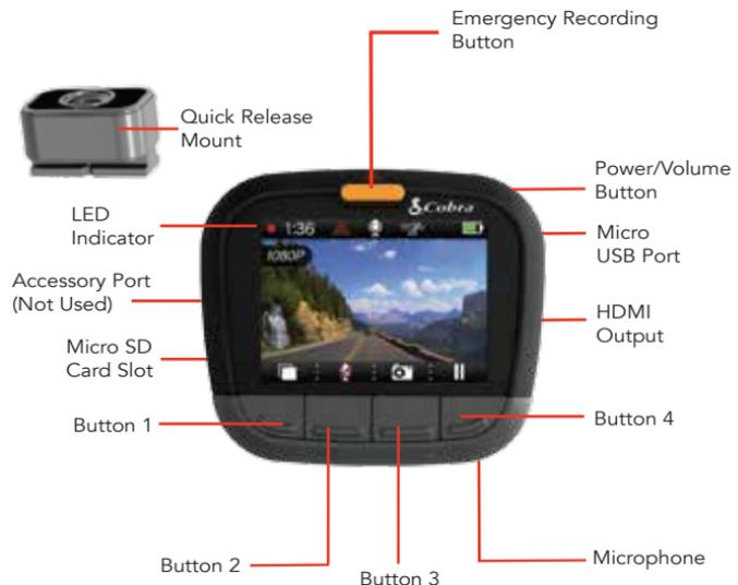
The functions of Buttons 1-4 are indicated by the icon directly above each button and change depending on the state of the unit.
