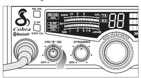
1 Rotate the **On/Off Volume** knob *clockwise* to turn unit on and adjust to a normal listening level.
