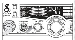
Full counterclockwise rotation opens the "gate" allowing all signals in.
