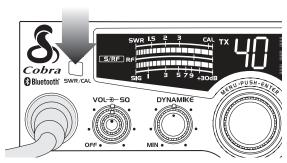
**1** The **S/RF-SWR-CAL** button must be in the S/RF mode.
