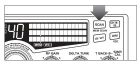
Pressing the Scan/Memory Scan button toggles from Off to Scan All Channels to Memory Channel Only Scan and back to Off.
