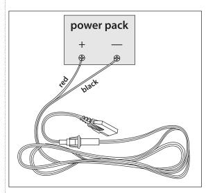
1 Simply connect the red (+) and black (-) leads of the transceiver to the corresponding terminals of the power pack.
