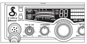
Attach the microphone cable to receptacle on front of unit and install unit in bracket securely.
