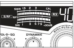
**1** The **S/RF-SWR-CAL** switch must be in the S/RF setting to read the meter.
