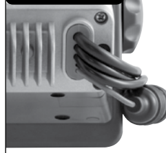
Wiring Located at Back of Radio
