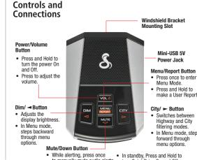
to manually mute audio alerts. turn Quiet Drive On and Off. In Standby and connected to
