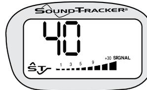
The INCOMING SIGNAL STRENGTH METER will be displayed when a signal is received.
