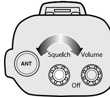
3 To achieve the Desired Squelch Setting (DSS), turn the Squelch control
