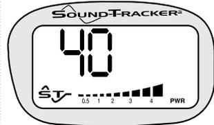
2 The TRANSMISSION POWER METER will be displayed when transmitting.
